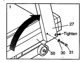
With the help of a second person, rotate the Left and Right Handrails (1, 11) up as shown. Insert two 3/8" x 1 1/4" Bolts (13) into the Left and Right Uprights (19, 27) and tighten the Bolts with the 7/32" Allen Wrench (90).
